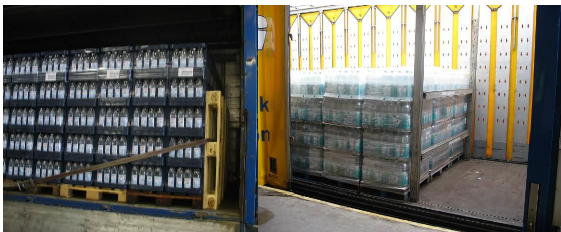
Fig. 6 & 7: Head lashing for securing to the rear and clamping bar systems
