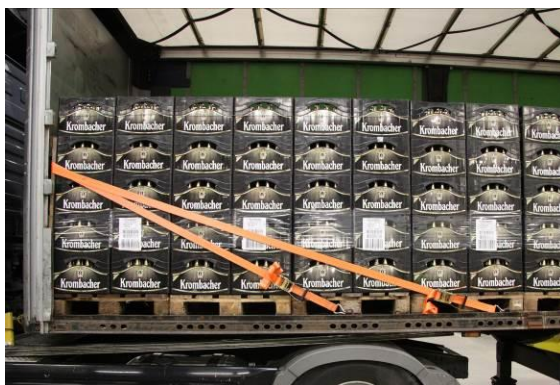
Fig. 3: Securing the front wall
