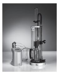
7-4425-00 CO2-Determination acc. to Blom-PU-002 incl. pump
