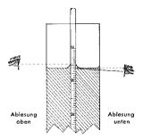
Standard-saccharometer for general malt analysis, 380 mm long, with thermometer scale ranging from 5 to 30°C and temperature correction table for cylinder No. 3-2000-30 or 3-2100-20
