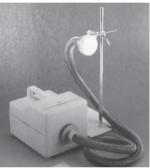
complete anaerobic system for germination of max. 11 Petri-dishes and/or 13 tubes, approx. 28 cm height, approx. 17 cm  $\varnothing$
